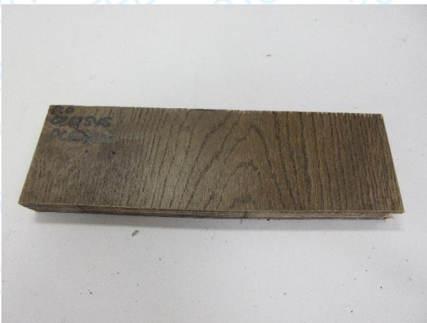
Tierdrylay magnetic wooden flooring. Engineered board with Oak wear layer. UV Oil Finish
