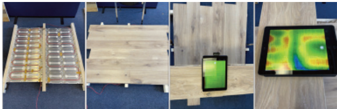
Left hand side of the testing rig 10T cable @ 10cm loops (See first picture)
